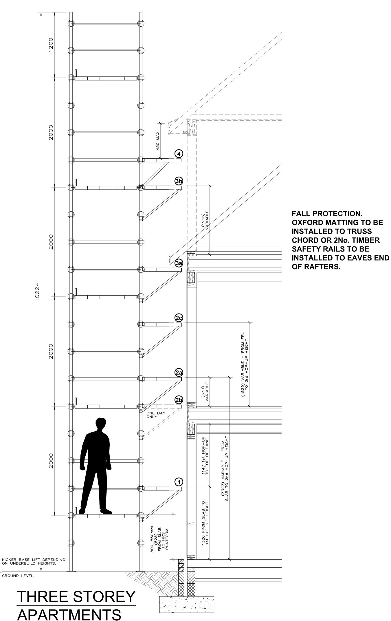
**FALL PROTECTION. OXFORD MATTING TO BE INSTALLED TO TRUSS CHORD OR 2No. TIMBER** SAFETY RAILS TO BE
